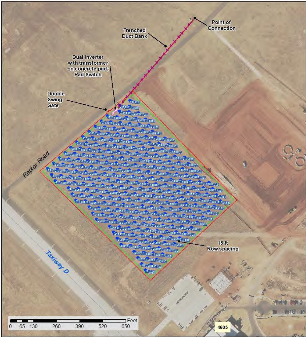
Figure 5. Proposed Solar PV Array at Site 3
